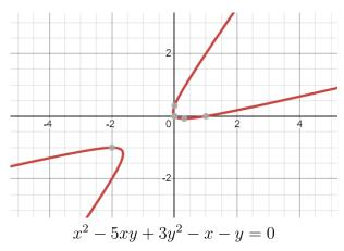
There are a few interesting subclasses of these PDEs depending on whether  $B^2 - 4AC$  is greater than, less than, or equal to 0. Informally, the names are based on how these equations look after taking what is known as a Fourier transform. If  $B^2 - 4AC > 0$ , for example, the PDE is **hyperbolic**. A guide image for this is to the left. If  $B^2 - 4AC = 0$ , the PDE is **parabolic**, while if  $B^2 - 4AC < 0$ , the PDE is **elliptic**.
